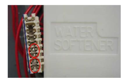
Or, the coils can be checked with a multimeter at the water softener itself.
